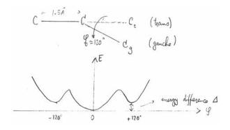
For  $(CH_2)^N$ ,  $\Delta$  is quite small (roughly 500 cal/mole or  $1/3k_BT$ ), and the polymer is very flexible at room temperature. For other polymers  $\Delta > k_BT$ , and gauche states with probability
