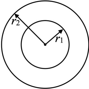
$$F_\nu(r_1) \times 4\pi r_1^2 = (dE_\nu)_1 = (dE_\nu)_2 = F_\nu(r_2)^2 \times 4\pi r_2^2 \quad (3)$$
