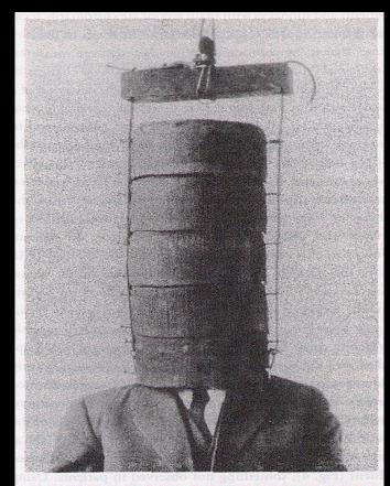
Fig. 1 Size matters. Early attempts to induce phosphenes by brain stimulation suffered from the difficulties of producing the requisite large, rapidly-changing electromagnetic fields. Here we see the arrangement of coils used by Magnussen and Stevens<sup>8,9</sup>. Coils were piled upon one another to create the increase in field strength. (Reproduced, with permission of Taylor & Francis, from the Philosophical Magazine, Ref. 8.)
