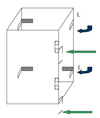
held together by small Hinge screws and glue gun glue at all joints points of contact
