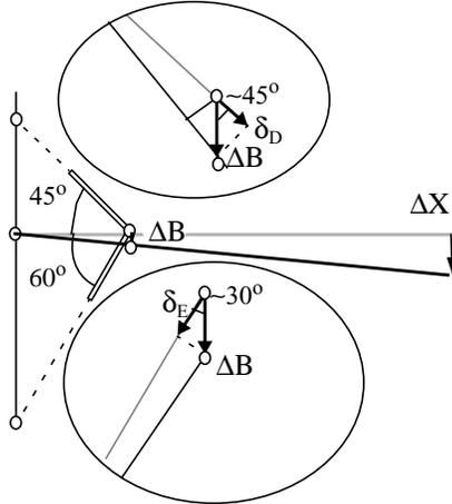
The deformations of member  $BD$  and member  $BE$  are related. How they relate is not obvious. We draw a picture, attempting to show the motion of the system from the undeformed state ( $W=0$ ) to the deformed state, then relate the member deformations to the displacement of point  $B$ .
