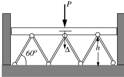
**5.13** A rigid beam is constrained to move vertically without rotation. It is supported by a simple truss structure as shown in the figure. The truss members are made of aluminum ( $E = 10.0 E+06 \text{ psi}; = 70 \text{ GPa}$ ). Their cross sectional area is  $0.1 \text{ in}^2 = 0.0645E-03 \text{ m}^2$ . The system bears a concentrated load  $P$  at mid span. The height of the platform
