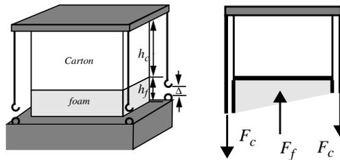
We begin by making a cut through the body to get at the internal forces in the cords and in the foam. We imagine the cords hooked to the floor; the system in the deformed state. We cut through the foam and the cords at some quite arbitrary distance up from the floor. Our isolation is shown at the right.
