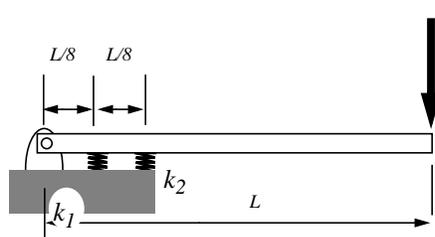
**5.11** The rigid beam is pinned at the left end and supported also by two linear springs as shown.
