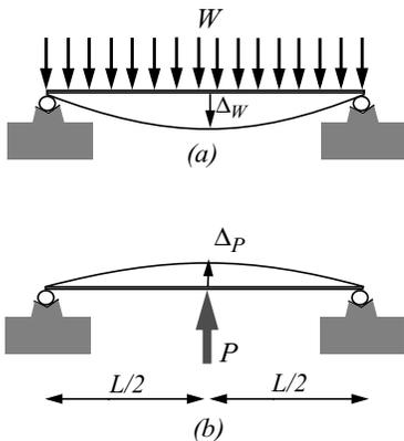
Forget the spring for a moment. Picture the beam as subjected to two different loadings: The first, a uniformly distributed load, figure (a); the second, a concentrated load  $P$  at midspan, as shown in figure (b), due to the presence of the spring.
