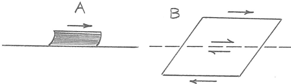
Figure 10-4. A) Shearing a thick telephone book. B) Shearing a continuous medium. The dashed line through the medium represents an imaginary plane of shearing. The single-barb arrows represent the friction force exerted by the material on one side of the plane on the material on the other side.
