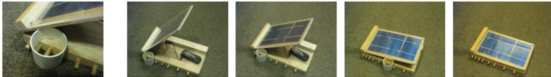
*Fig. 6: Notch and Wedge Adjustment System*
