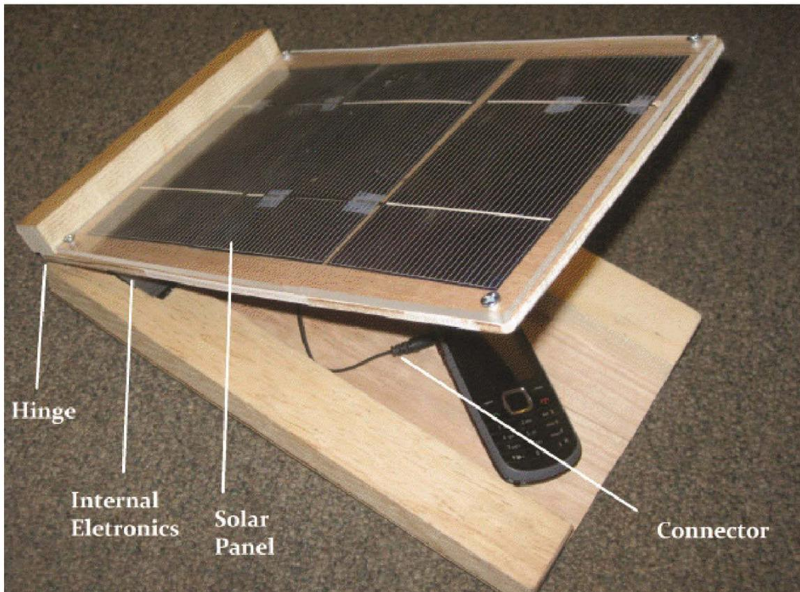
Our final design (see above) incorporates our design specifications to the greatest extent possible. Its cost has been maintained at just over the \$20 specified (see below) through the use of low-cost and locally available materials. For instance, protoboards are not
