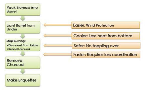
Figure 13 – Parts of the charcoal making process that we were able to improve
