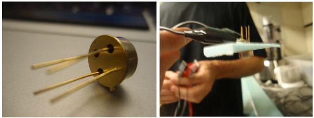
Figure 5 – Left: TPS 334 Thermopile; Right: Thermopile mounted on foam and connected to voltmeter
