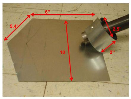
Figure 9 – Final product: pentagonal metal seal w/ cylindrical handle
