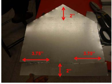
Figure 10 - Metal seal w/ measurements before handle is constructed
