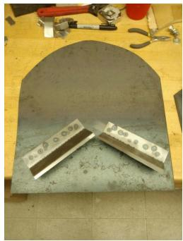
**Figure 4** - Plate with a spot-welded handle that sits 45 deg. to the plate, with a semi-circular edge. <u>3. Heat Insulation Testing</u>
