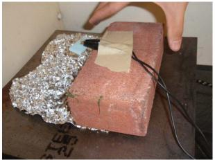
**Figure 6** - Thermopile setup mounted to brick and set over very crinkled foil; entire setup on top of hotplate
