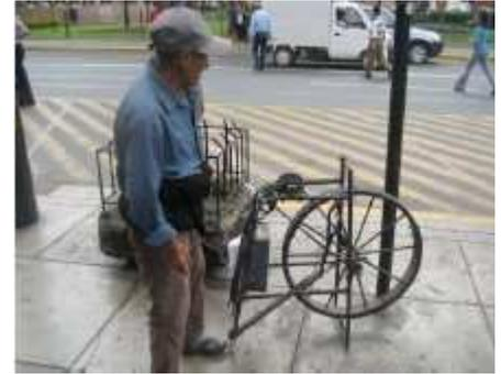
A portable pedal-powered grinding wheel
