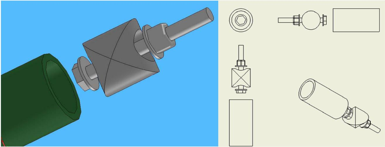
**Figure 14: Second Alignment Assembly.** This assembly requires only six pieces and can be easily tightened before positioning within the pylon. We plan to test the effectiveness of larger versions of the assembly this summer.
