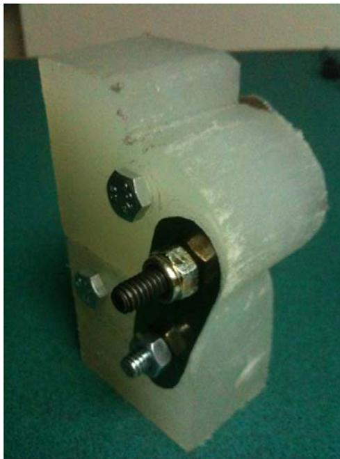
***Figure 1: Prototype of Single Four Bar Linkage.*** This prototype is a rough model used to better conceptualize the costs and benefits of using a knee with a single four bar linkage. It was manufactured using solely a band saw, power sander, and drill press. The prototype is based on the work of the Stanford team, following the polycentric design with similar measurements.
