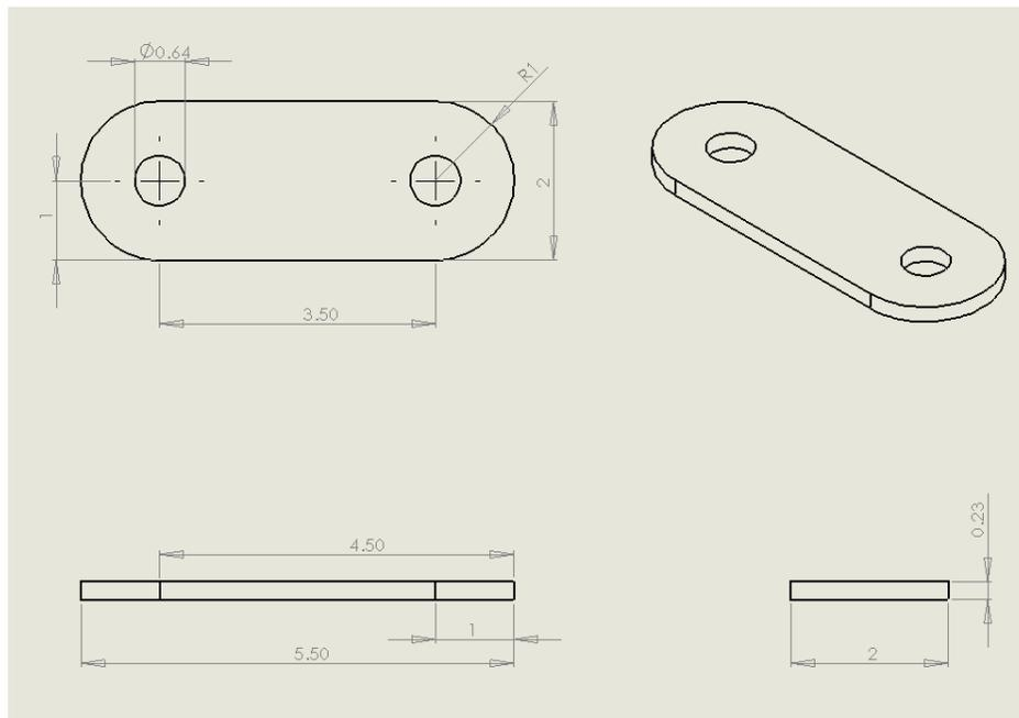
**Figure 5: Smaller Knee Linkage.** This smaller linkage was created similarly to the large one. It is placed on the back left side of the knee when viewed head on, as shown in Figure 6.
