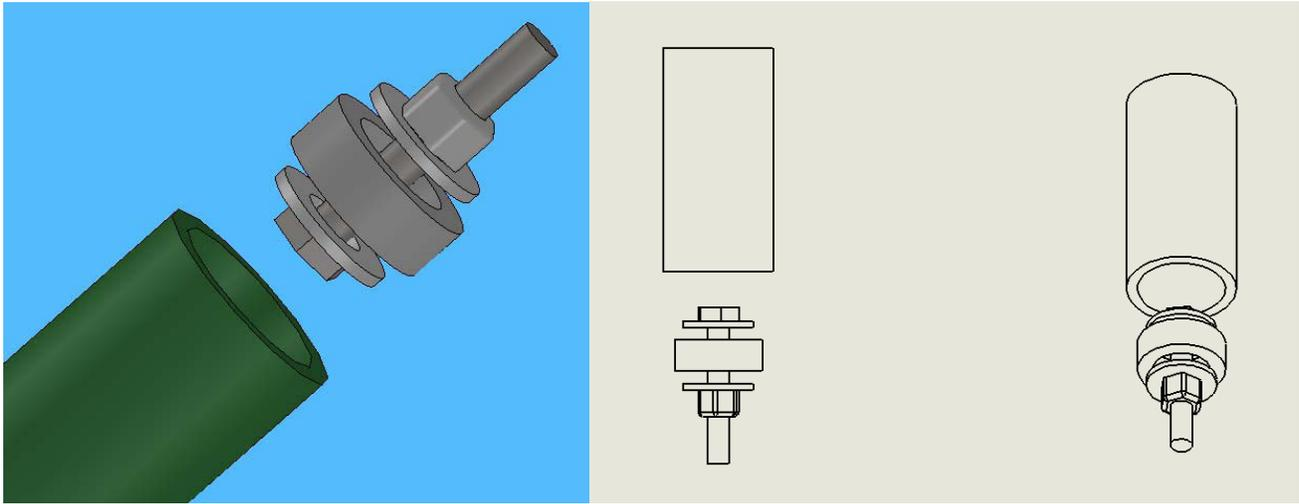
**Figure 11: Initial Alignment Assembly.** Shown here is the completed assembly for the initial knee alignment system. It is created from a ring of plastic, two washers, and a nut and bolt.
