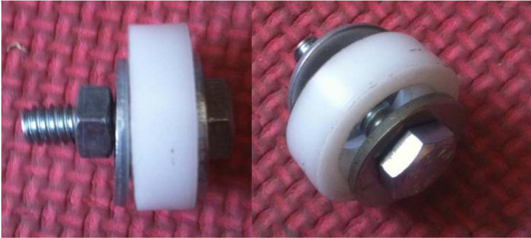
**Figure 11: Initial Alignment System.** In the alignment system pictured here, a short ring of Delrin is used to support a moveable bolt, which is to be screwed into the top of a prosthetic knee joint. The alignment system is then tightened in the desired position and fastened to the end of a pylon.
