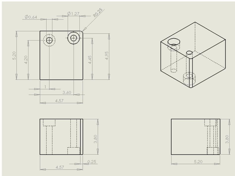
**Figure 3: Bottom Portion of Single Linkage Knee.** Shown here is a three-section view of the knee's bottom portion. The accompanying physical part was manufactured via the same processes as the knee's upper portion.
