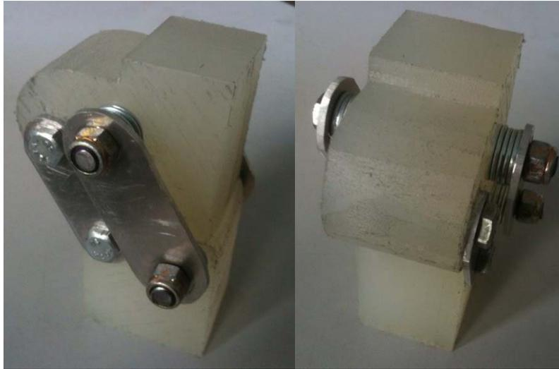
**Figure 7: Prototype of Multiple Linkage Knee.** This knee was manufactured similarly to the single linkage knee. The primary differences were adding twenty thin washers for spacing, changing the linkages to aluminum, and including only two countersunk holes.
