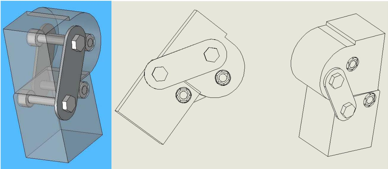
**Figure 6: Completed Assembly for Single Linkage Knee.** This assembly includes two high-density polyethylene blocks, two steel linkages, four bolts, and four lock nuts. The pieces to be manufactured are described in Figures 2 through 5.
