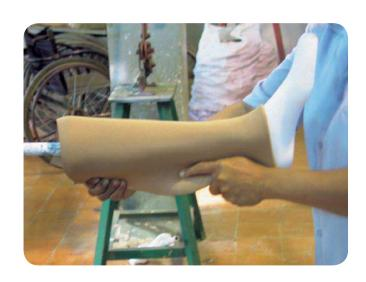
Cut off the excess with a cutter or a pair of scissors.
