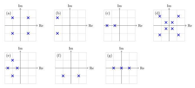
(b) Assume all the pole diagrams are on the same scale, which of the stable systems decays to equilibrium the fastest.
