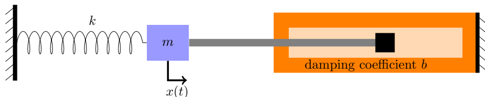
Spring-mass-damper with no outside force
