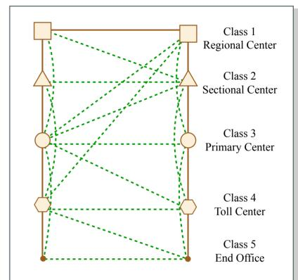
Five-level toll switching plan in use from the 1950s. A variety of routings was possible with a maximum of nine trunks in tandem.
