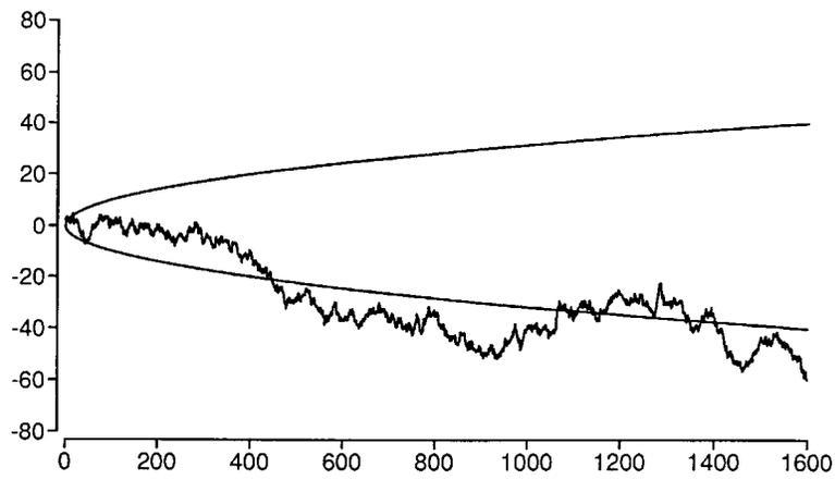
Figure 11.8: Waveform of discrete-time Wiener process with  $\sigma = 1$ . Smooth lines show  $\pm 1$  standard deviation
