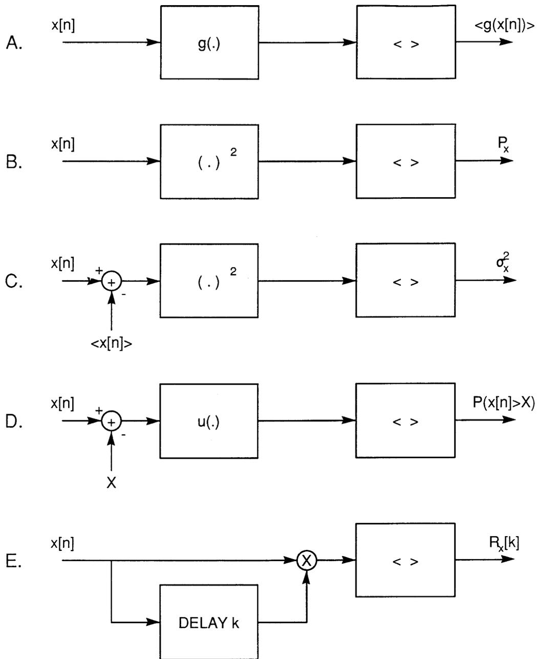
Figure 11.1: Computation of time averages of random signals. A. Average of a memoryless function  $g(x[n])$ . B. Mean Power. C. Variance. D.  $P(x[n] \geq X)$ . E. Autocorrelation function.
