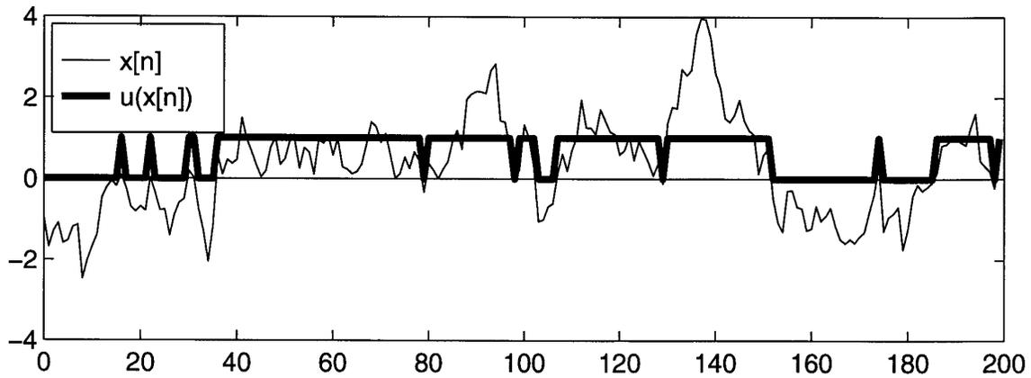
Figure 11.2: Use of step function  $u(x[n])$  in computing  $P(x[n] \geq 0)$ .
