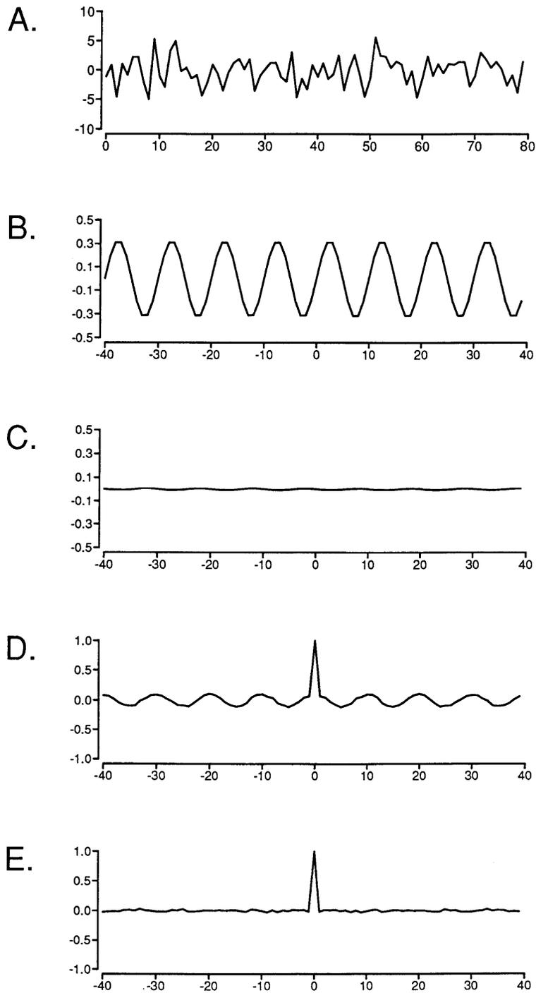
Figure 11.5: A. Waveform of a sine wave buried in additive, white noise. B. Estimated cross-correlation function between the signal in A. and the unit cosine. The estimate is based on 4000 samples. C. Cross-correlation between white noise and unit cosine. D. Estimated autocorrelation function for the signal in A. E. Autocorrelation function of the white noise.
