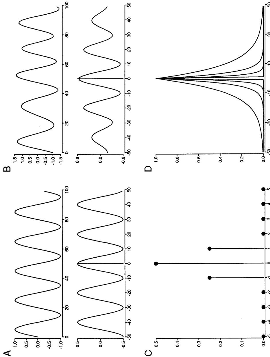
Figure 11.4: A. Waveform and autocorrelation function of the sine wave  $\sin(0.1\pi fn)$ . B. Same as in A. for the three component signal  $\sin(0.1\pi fn) + 0.5 \sin(0.08\pi fn) + 0.5 \sin(0.12\pi fn)$ . C. Autocorrelation function of the FIR filter  $y[n] = 0.5(x[n] + x[n - 1])$  for white noise input. D. Same as in C. for first-order recursive filter  $y[n] = ay[n - 1] + x[n]$ . The autocorrelation function is shown for  $a = 0, 0.5, 0.75, 0.9$ .
