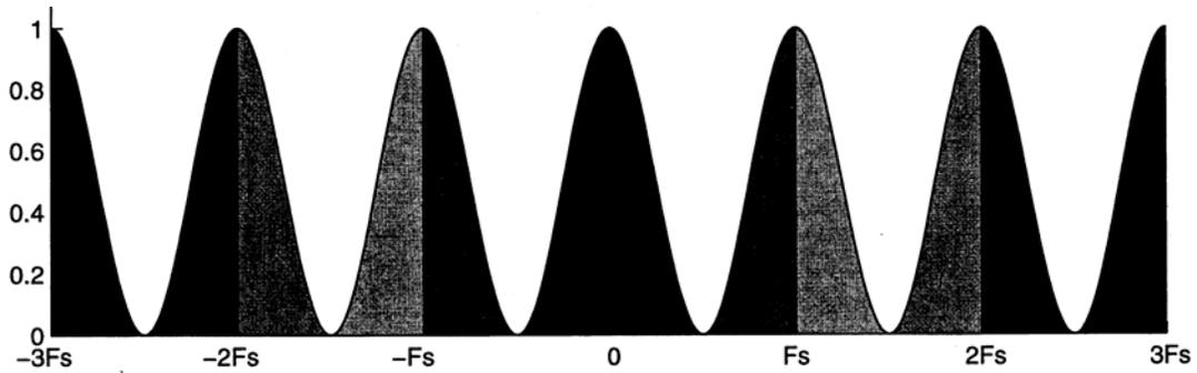
Figure 1.15: Sampling of a bandlimited signal,  $F_s = 2W$
