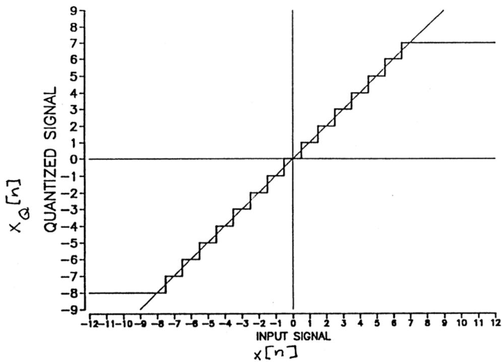
Figure 1.8: Input-output function for a 4-bit quantizer.
