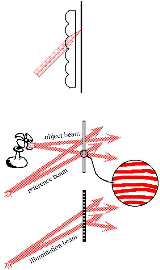
impinge on the film at different angles; each of these produces its own interference pattern, creating superimposed picket-fence patterns of different rotations and spacings.
