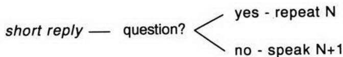
Figure 9.14. Grunt analyzed short utterances to detect whether they might be questions and reacted accordingly.
