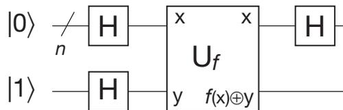
Fig. 11: Circuit implementing the Deutsch-Jozsa algorithm.
