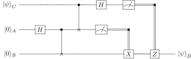
Fig. 10: Circuit for teleportation: the qubit  $|\psi\rangle_C$  (initially in Alice's hands) is teleported to Bob ( $|\psi\rangle_B$ ) by using two qubits in a Bell pair  $|\Phi\rangle_{AB}^+$ .
