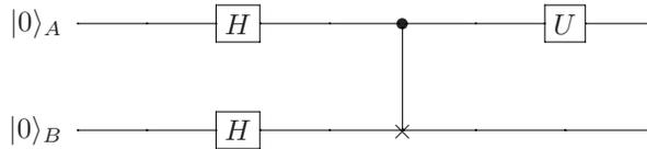
Fig. 9: Quantum circuit, showing Hadamard, CNot gate and a general gate  $U$
