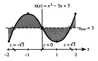
In this sketch it is easy to see that the two shaded areas above the dotted line fit into the shaded areas below the line. The area under the curve equals that of a rectangle whose height is the average value.
