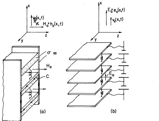
Fig. 8.8.1. One-dimensional compressional motions. (a) Magneto-acoustic waves in perfectly conducting liquid across uniform magnetic field. (b) electro-acoustic waves in potential conserving continuum along uniform electric field. Lumped models emphasize salient features of dynamics.
