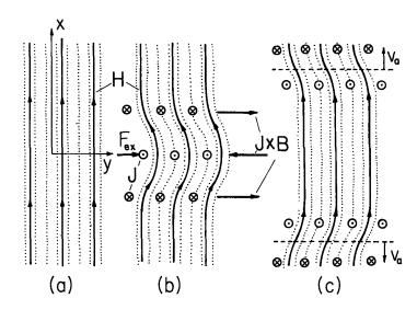
Fig. 8.6.1. (a)Perfectly conducting fluid initially at rest in uniform magnetic field.
