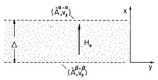
Fig. 8.6.2. Layer of liquid metal or plasma with ambient magnetic field  ${\rm H}_{\rm O}$ .
