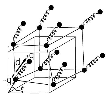
Fig. 2.8.1. Model for dipoles fixed to deformable material. The model pictures the negative charges as fixed to the material, and then the positive halves of the dipoles fixed to the negative charges through internal constraints.
