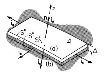
Fig. 2.10.1. Volume element enclosing a boundary. Dimensions of area A are much greater than  $\Delta$ .
