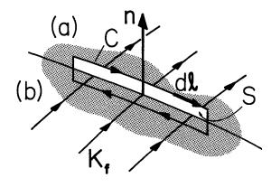
Fig. 2.10.3. Contour of integration C enclosing a surface S that intersects the boundary between regions (a) and (b).
