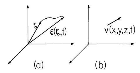
Fig. 2.4.1. Particle motions represented in terms of (a) Lagrangian coordinates, where the initial particle coordinate  $r_0$  designates the particle of interest, and (b) Eulerian coordinates, where (x,y,z) designates the spatial position of interest.
