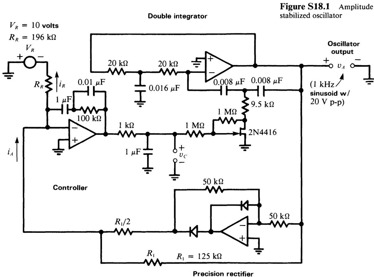
Now, as shown in Figure S18.1, we use the same FET circuit as in Figure 12.4, including the 9.5 k $\Omega$  resistor, so that nominally  $R/2 = 10$  k $\Omega$ . (Thus,  $R = 20$  k $\Omega$ .) Then, all the equations describing the FET in Section 12.1.4 apply. Specifically, from Equation 12.23
