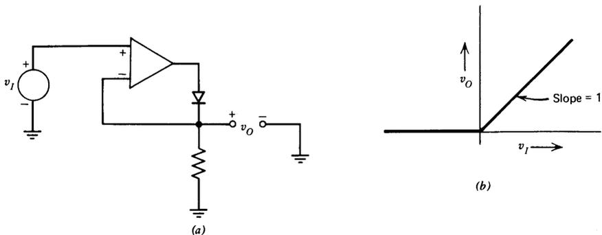
**Figure 11.18** Precision rectifier. (a) Circuit. (b) Transfer characteristics.
