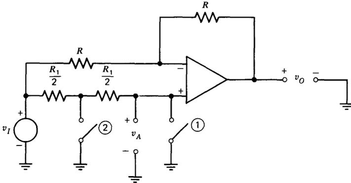
**Figure 11.33** Amplifier that provides gain of  $\pm 1$ .
