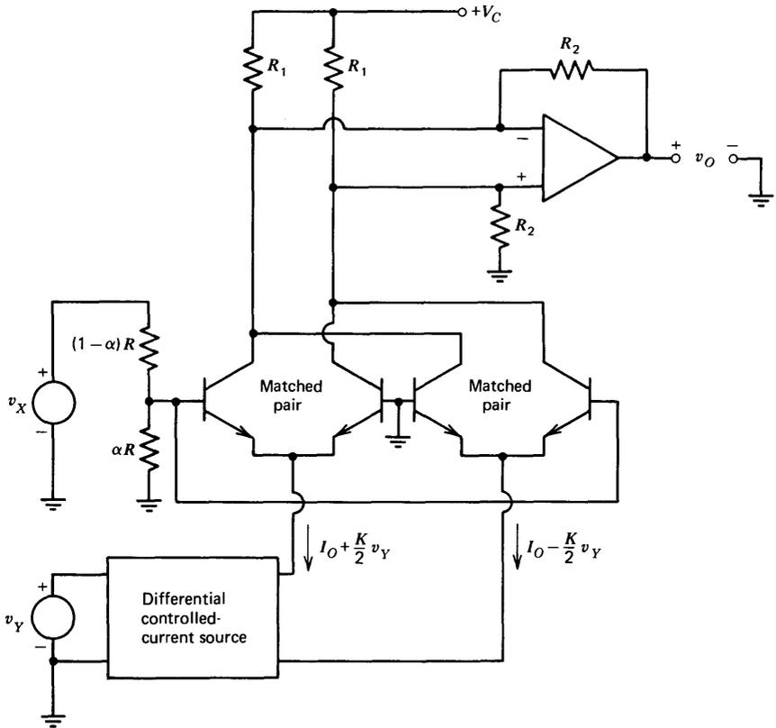
**Figure 11.29** Four-quadrant transconductance multiplier.
