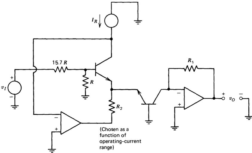
Figure 11.27 Antilog circuit.
