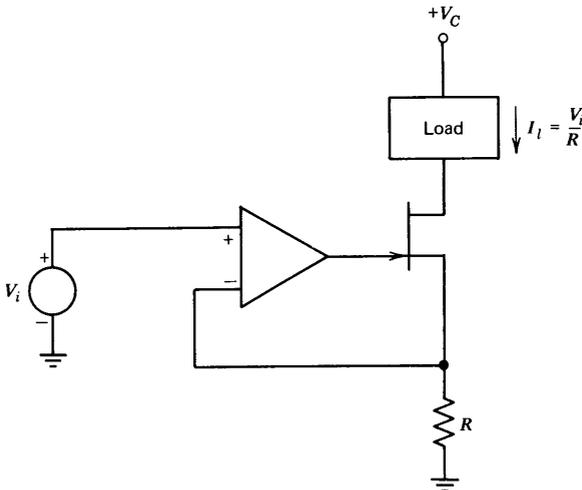
**Figure 11.14** Current source using a field-effect transistor.
