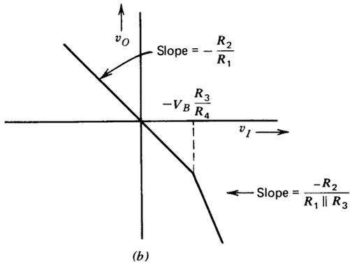
**Figure 11.24** Expander. (a) Circuit. (b) Transfer characteristics.
