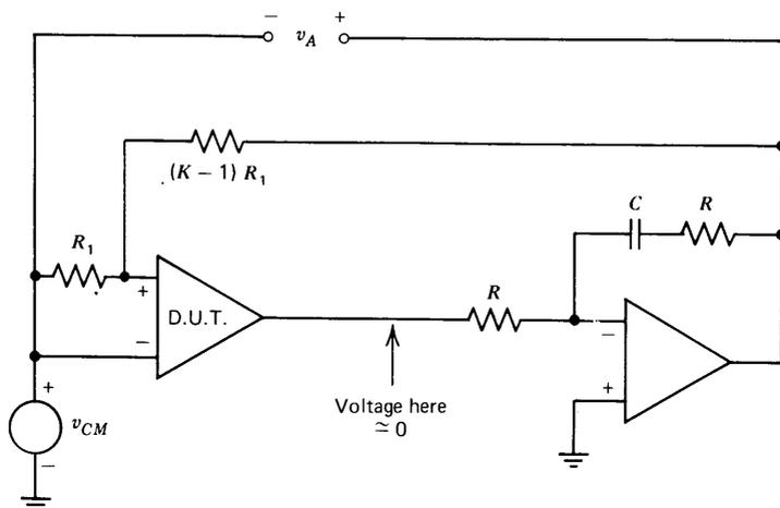
**Figure 11.4** Circuit for measuring common-mode rejection ratio.
