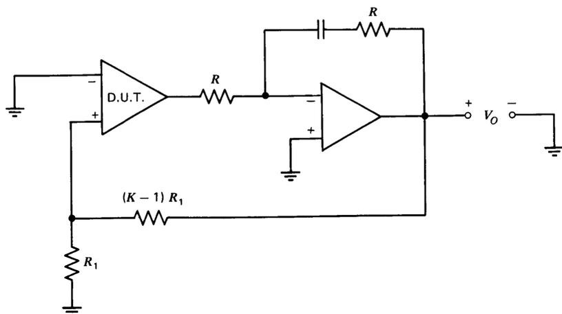
**Figure 11.3** Offset-measurement circuit with increased loop transmission.
