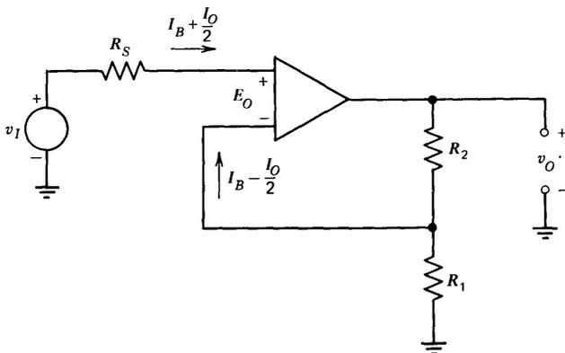
Figure 11.1 Noninverting amplifier.
