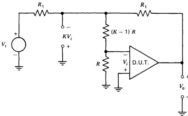
**Figure 11.5** Connection for measuring the open-loop transfer function.
