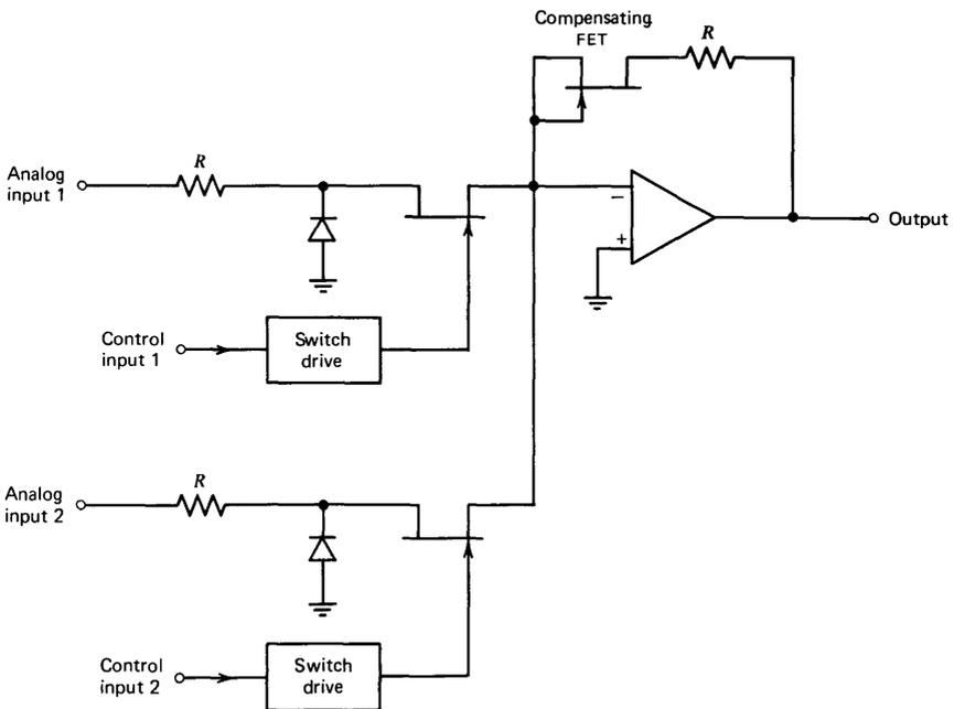
**Figure 11.31** Inverting multiplexer.
