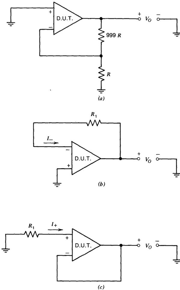
**Figure 11.2** Circuits used to determine offset voltage and input currents. D.U.T. = Device Under Test. (a) Measurement of offset voltage. (b) Measurement of  $I_-$ . (c) Measurement of  $I_+$ .
