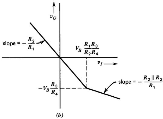
**Figure 11.22** Limiter. (a) Circuit. (b) Transfer characteristics.
