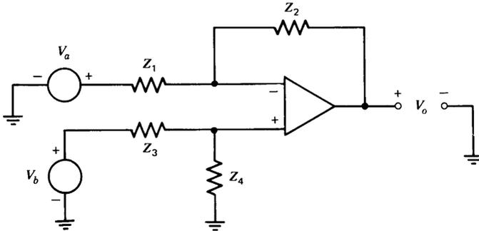
**Figure 11.10** Differential connection.
