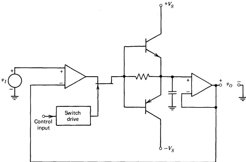
**Figure 11.34** Sample-and-hold circuit.
