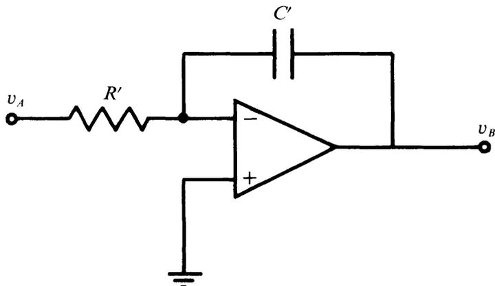
Using the results of Section 5.2.3, we can design a lag network with its pole at  $s = -1$  and its zero at  $s = -20$ . That is,  $\alpha\tau = 1$ , and  $\tau = 0.05$ ,  $\alpha = 20$ . This network appears as shown in Figure S17.3.
