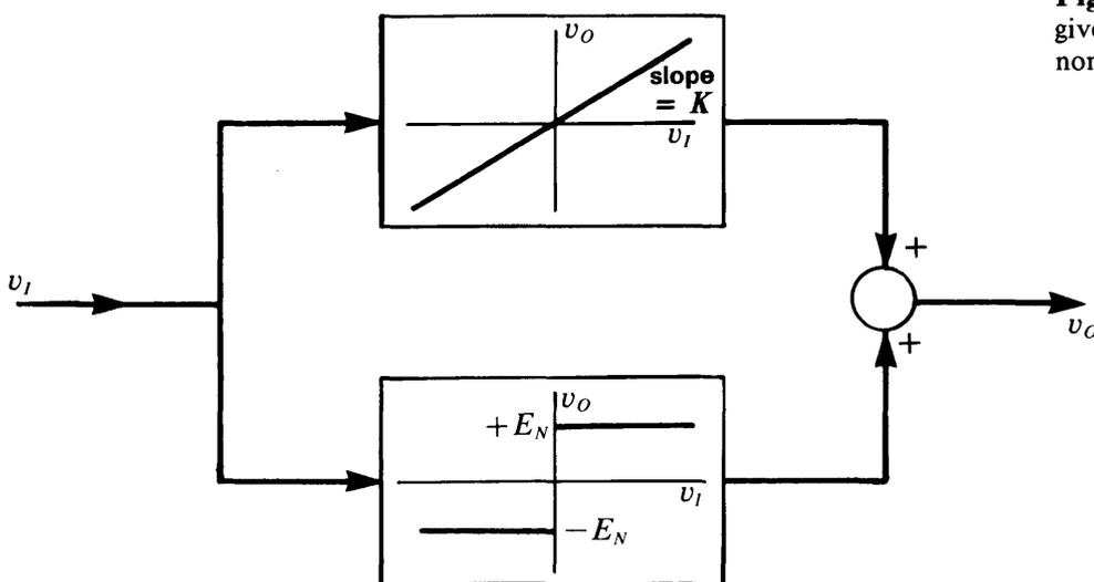
**Figure S15.1** Decomposition of given nonlinearity into two nonlinearities.
