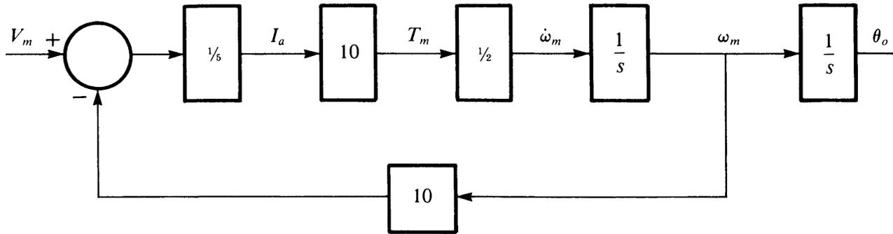
Lastly, we add the differential amplifier. With the error signal defined as in Figure 2.27, and an amplifier gain of 10, we have
