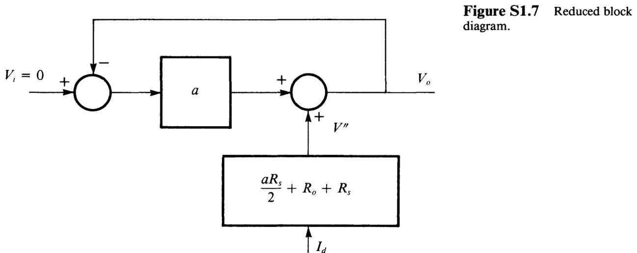
$$V_o = I_d \left( \frac{aR_s}{2} + R_o + R_s \right) \left( \frac{1}{1+a} \right) \quad (\text{S1.19})$$
