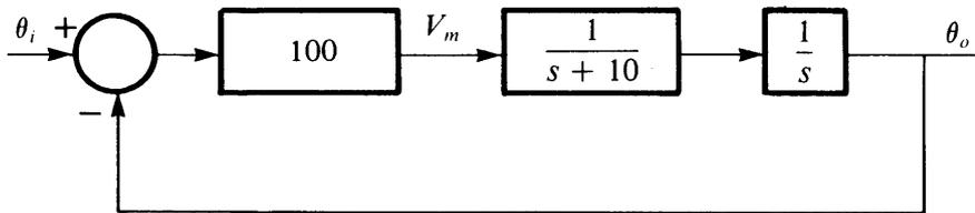
**Figure S1.12** Reduced antenna-rotator block diagram.
