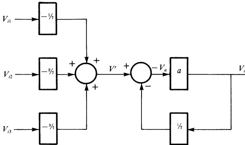
**Figure S1.2** Block diagram for three-input inverting amplifier.
