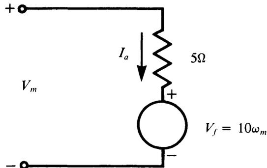
where  $\omega_m$  is the motor rotational speed in radians per second and  $V_f$  represents the motor's back e.m.f. voltage.
