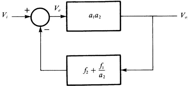
Figure S1.4 Reduced block diagram.
