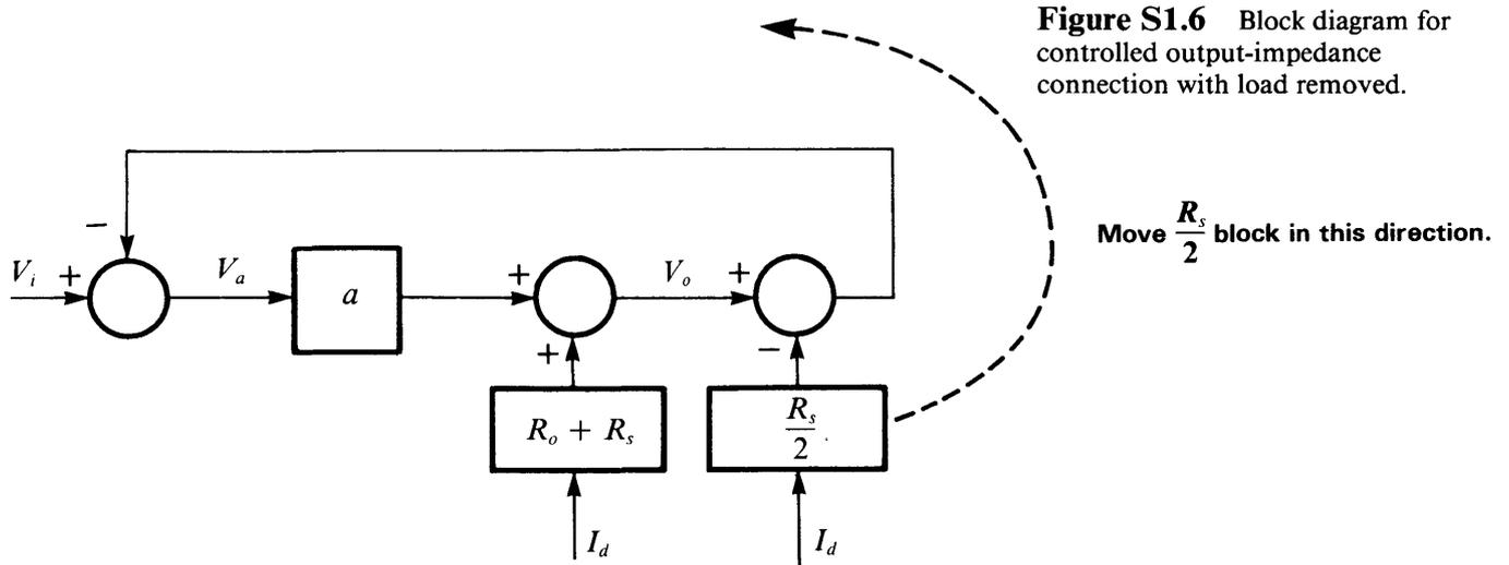
To calculate output-resistance  $R_{amp}$ , we need the ratio  $\frac{V_o}{I_d}$ . Note that  $V_i$  does not affect this ratio (as a consequence of linearity); thus, we set  $V_i = 0$ . We then manipulate the block diagram by propagating the  $\frac{R_s}{2}$  block forward around the loop, as indicated in Figure S1.6, to arrive at the reduced block diagram of Figure S1.7:
