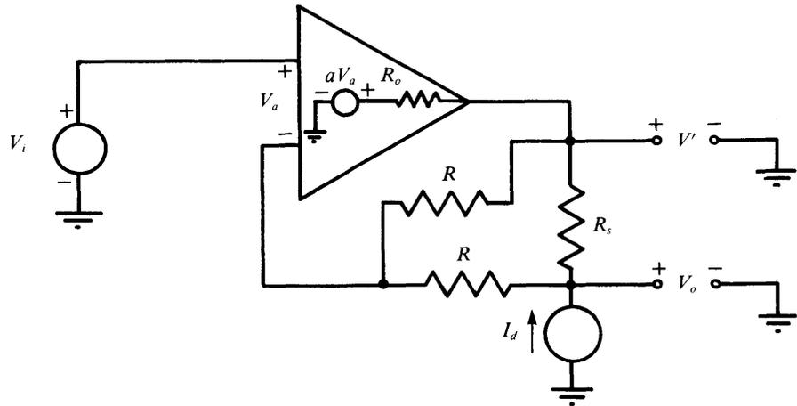
Because  $R \gg R_s$ , we assume that all of  $I_d$  flows through the series connection of  $R_o$  and  $R_s$ . Thus
