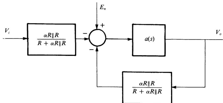
By a block-diagram manipulation, Figure S8.8 reduces to Figure S8.9.
