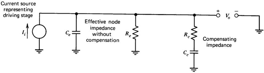
**Figure 8.4** Compensation by adding a shunt impedance.
