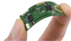
**electrodes:** etched on a flexible PCB
