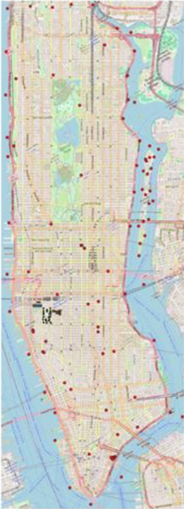
Figure 7 The well data (red dots) displayed were imported into PetraSim and used to create a geologic model of the entire Manhattan Island
