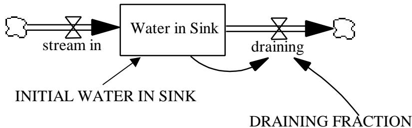
Figure 13: Vensim Equivalent of Figure 5: Model for draining sink with constant inflow
