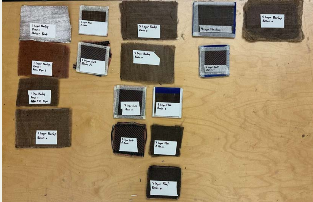
1 to 5 layers of Burlap, Flax, and Carbon Fiber Samples
