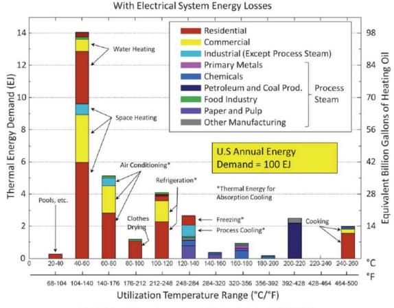
Fig. 1 Estimated thermal energy consumed in America below 260 °C (500 °F).
