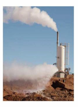
17 March 2008 --Wellhead flow rate 18 kg/s at 275 bar, 208°C and rising
