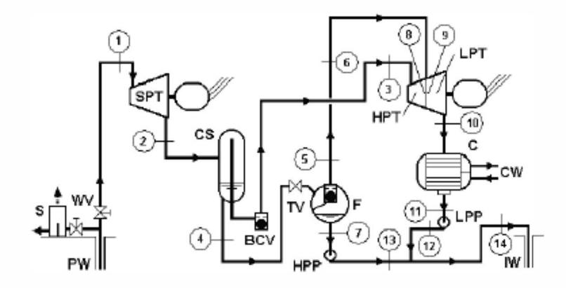
Trilateral supercritical vapor cycle
