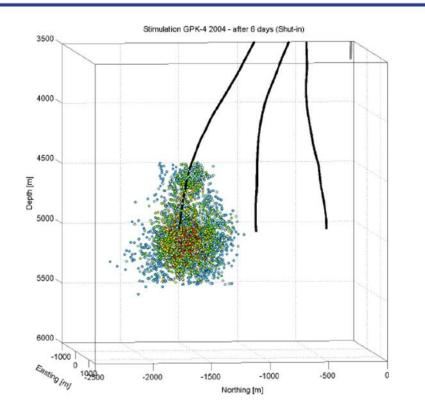
"snap shot" of microseismic events during hydraulic fracturing at Soultz from Roy Baria
