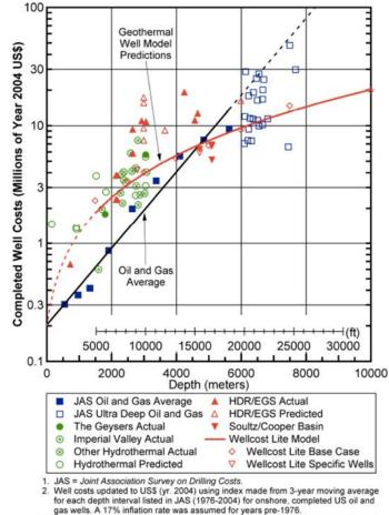
Drilling costs for geothermal wells compared to oil and gas wells
