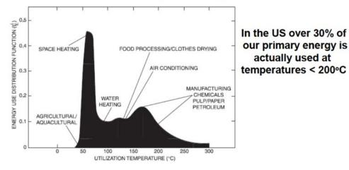
Figure 11.5. Fractional energy use distribution as a function of end-use temperature for non-electric applications below 300°C. The function  $f_E^i$  at  $T_i$  is simply the derivative of the cumulative energy use at that specific temperature  $T_i$ . Source: Tester (1982).
