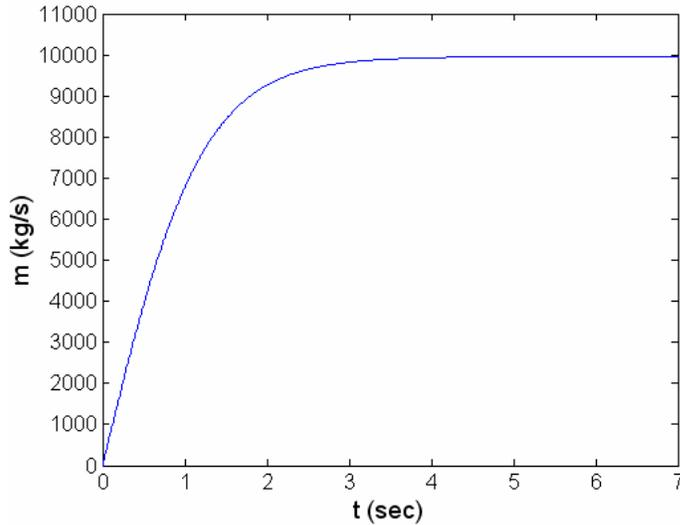
**Figure 1. PWR primary system mass flow rate during cold zero-power start-up.**
