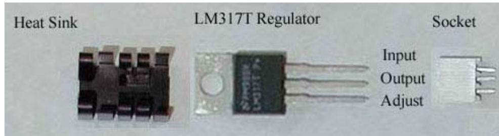
Figure 12: Heat sink, LM317T voltage regulator, and socket
