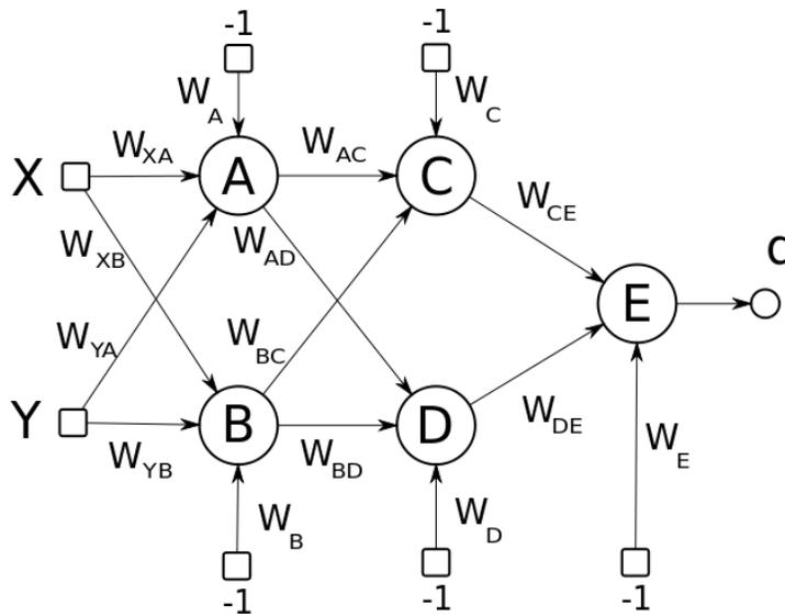
**B1. (9 points)** For the neural network, given above, where the sigmoid units use  $S_2$  and the performance function is  $P_2$ , write out the equation for  $\delta_E = \frac{\partial P_2}{\partial o_E} \frac{\partial o_E}{\partial z_E}$ . Express your answer in terms of  $d$ ,  $k$ ,  $s()$ , and  $z_E$  (the sum of weights times the inputs at node E). Hint:  $o_E = s(z_E) + s(z_E - k)$ .
