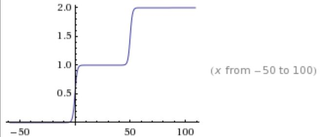
For instance, when  $k = 50$ , the sigmoid  $S_2(x)$  would have the graph shown at the right. Thus, the output is roughly, 0 when  $x$  is  $< 0$ , 1 when  $0 < x < 50$ , and 2 when  $x > 50$ . Changing the sigmoid function triggers a similar change in the performance function in order to normalize range of values of the error.
