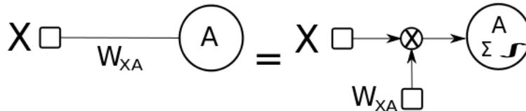
One possible method for making neural nets capable of multi-class classification is to change the sigmoid function. Inspired by the 6.034 GPA function, Yuan decides to adopt a 2-step sigmoid function as the output of the sigmoid unit, creating neural nets that can output roughly 3 values, 0, 1, and 2. The 2-step sigmoid  $S_2(x)$  has the following equation.
