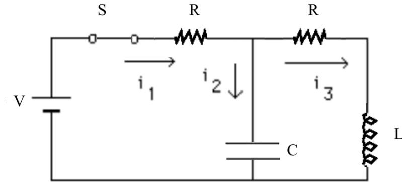
(a) Using Kirchoff's Loop Rule as modified for inductors, what is the sum of the potential drops around the outer loop (the loop including both the emf and the inductor) if we move clockwise around the loop?
